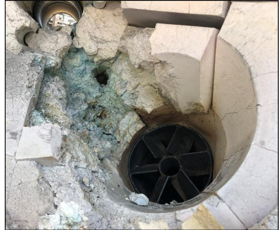
Early failure of zirconia lining due to injector mis-alignment
